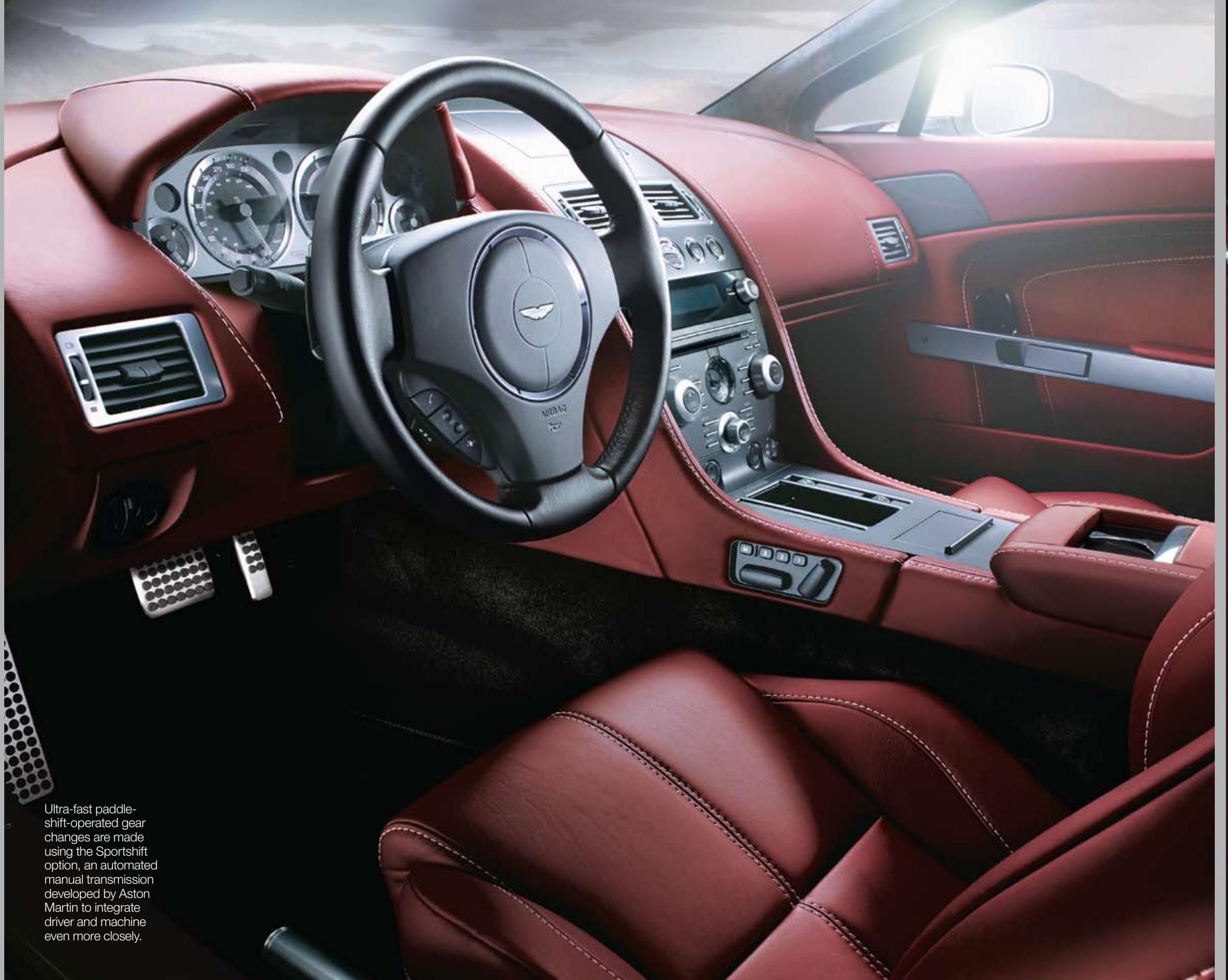
Ultra-fast paddle-shift-operated gear changes are made using the Sportshift option, an automated manual transmission developed by Aston Martin to integrate driver and machine even more closely.
